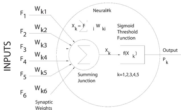
Fig. 3. Neuron computation structure.
