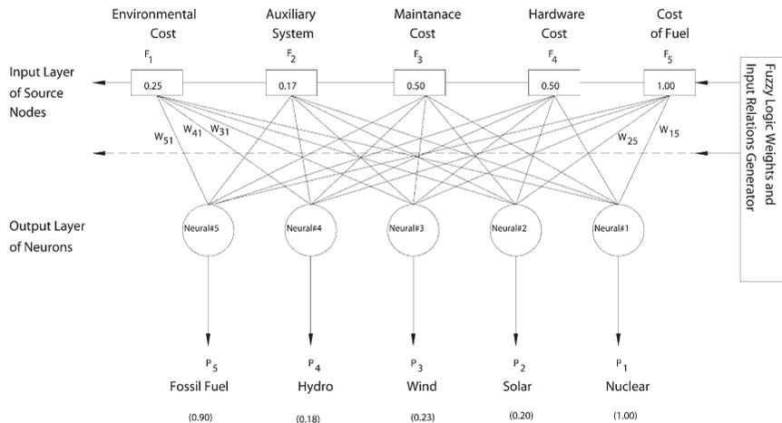
Fig. 4. Neuro-fuzzy network to make decision on best system based on cost factors.
