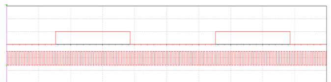
Figure 10: Input (down) and output (up) pulses of frequency divider
