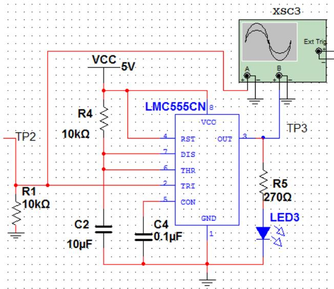
Figure 5: Fixed duration pulse generator
