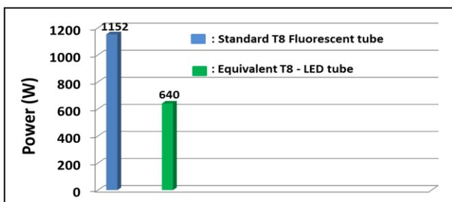
Figure 11: Power consumption data per lighting units in a class room
