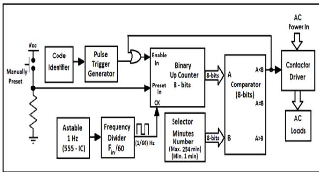
Figure 1: Main block diagram of the proposed energy saver
