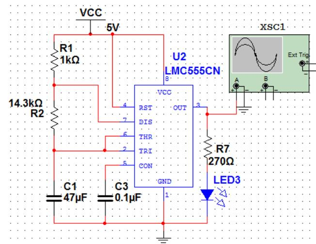
Figure 7: Astable multivibrator-1 Hz
