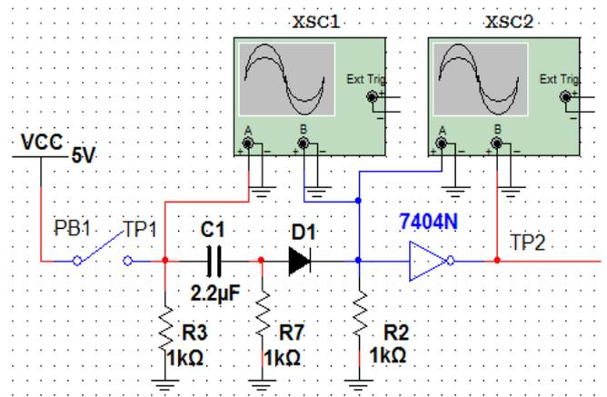
Figure 3: Differentiator circuit
