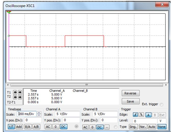
Figure 8: Astable multivibrator-1 Hz output pluses
