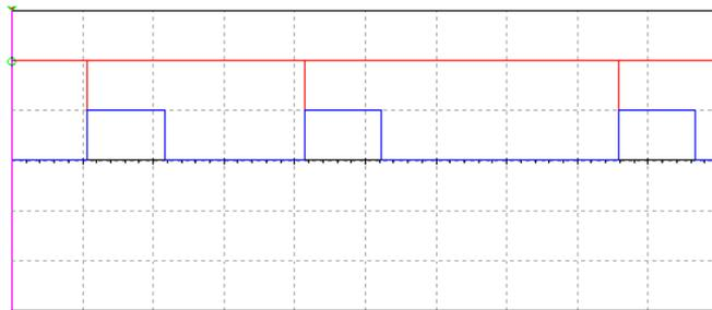
Figure 6: Trigger pulse TP2 – red color, and fixed duration pulses TP3 – blue color
