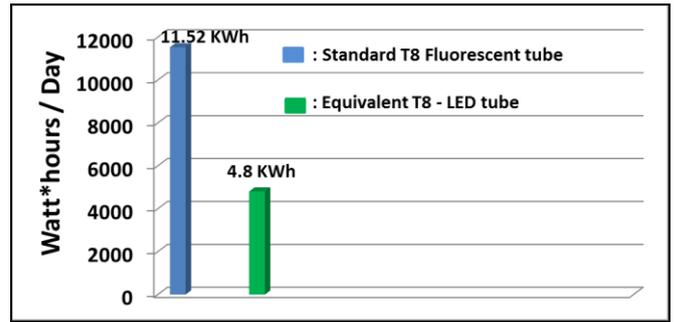
Figure 12: Total KWh/day of the lighting system in a class room without (blue bar) with (green bar) of the proposal of this study
