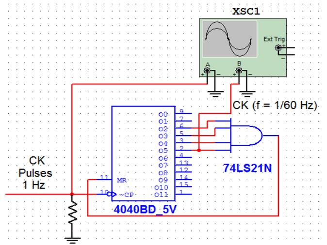
Figure 9: Digital frequency divider with division rate (1/60)
