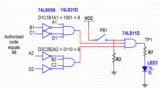
Figure 2: Code identifier circuit (Activated code = 96)
