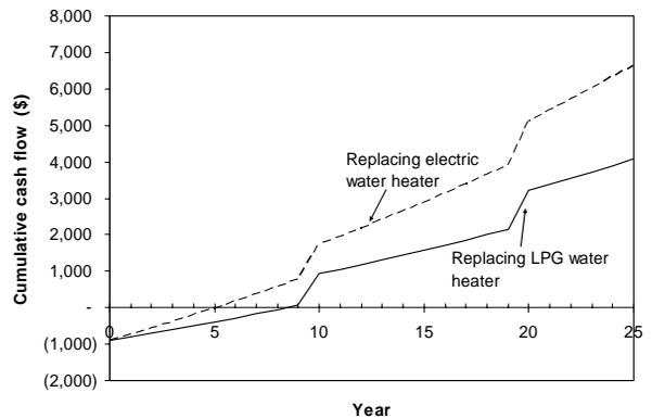
Fig. 7 Cumulative cash flow for SWH replacing electric and LPG heaters
