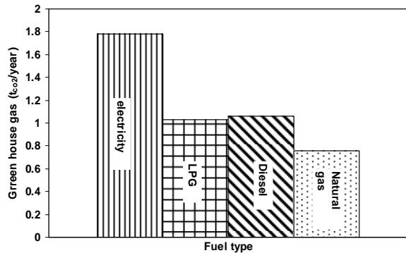
Fig. 6 Reduction in GHG emission when replacing conventional water heaters with SWH
