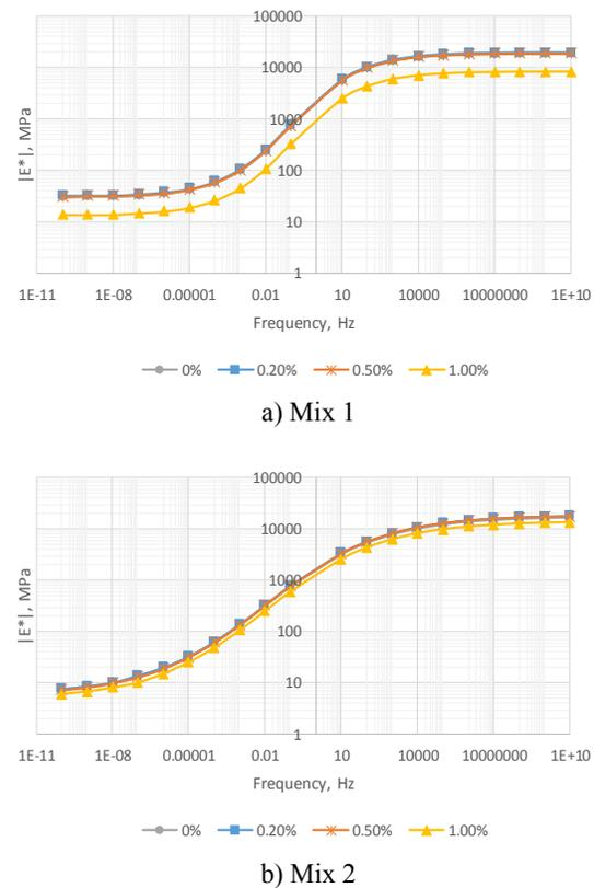
Figure-2. Master curves for asphalt mixes.
