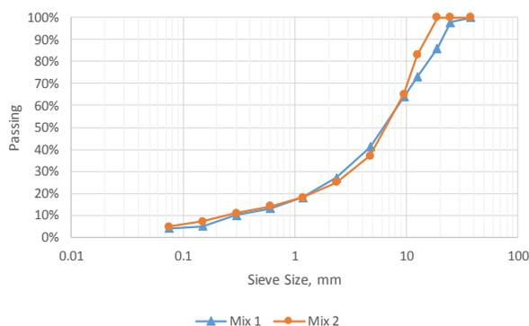
**Figure-1.** Aggregates gradations for Mix 1 and Mix 2.
