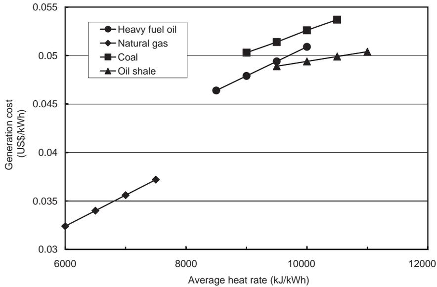
Fig. 5. Effect of variation in heat rate on levelised generation cost for various power plants.
