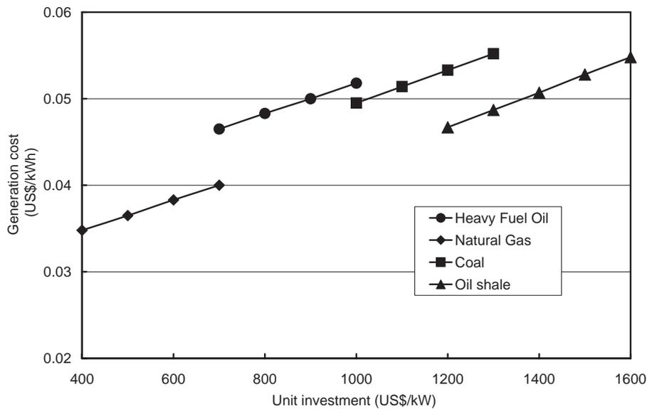
Fig. 2. Levelised unit electricity generation cost variation with respect to unit investment.
