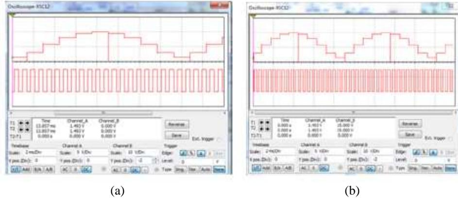
Figure 9. (a) Output Waveform of the Frequency Divider and Reference Signal Generator at Half of Maximum Reference Frequency Value, (b) Output Waveform of the Frequency Divider and Reference Signal Generator at Maximum Reference Frequency Value
