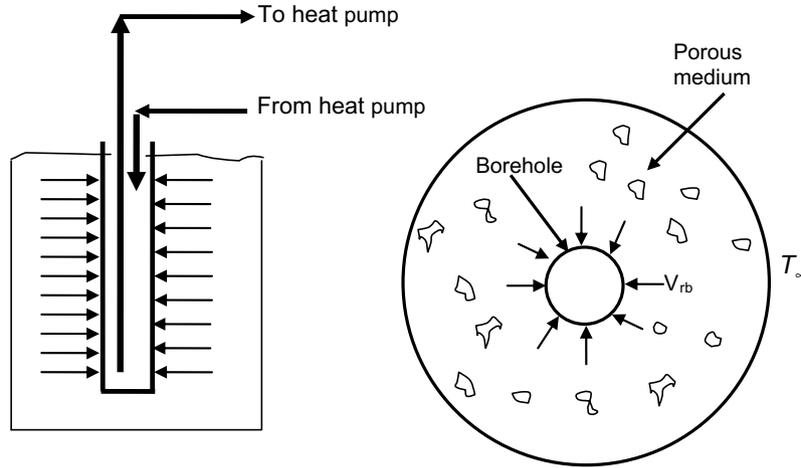
Fig. 4. One-dimensional model for the standing column well.
