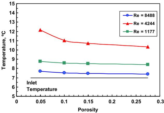
Fig. 11. Variation of the outlet temperature with the porosity.
