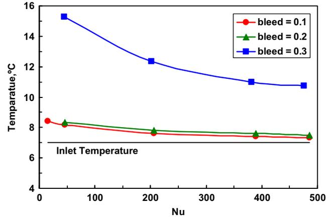
Fig. 12. Effect of Nusselt number on the outlet water temperature.
