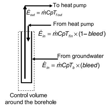
Fig. 6. The energy balance in the borehole model.
