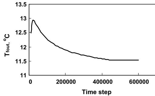
Fig. 7. Steady-state condition for water outlet temperature and time steps.
