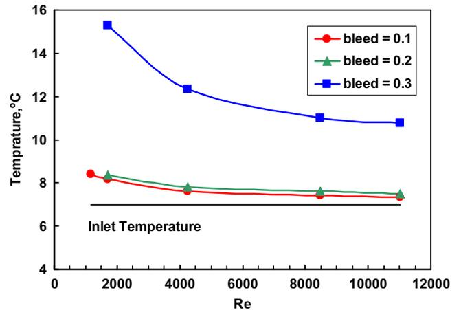
Fig. 8. Variation of the outlet temperature with Reynolds number.
