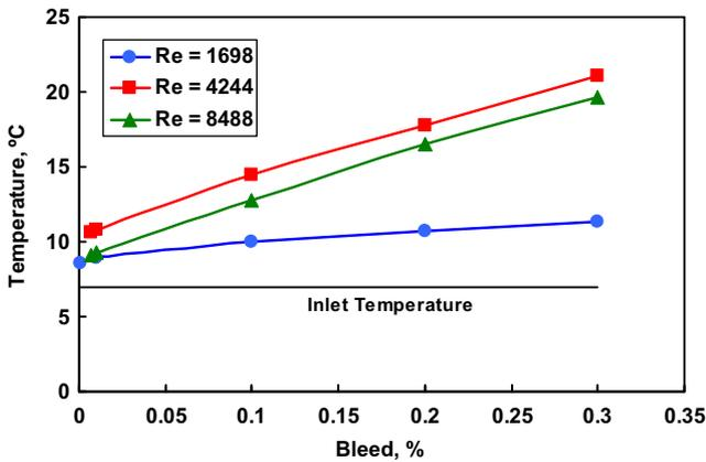
Fig. 10. Variation of the outlet temperature with the percentage of bleed.
