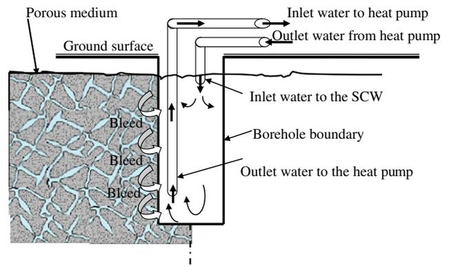
Fig. 1. Schematic diagram of the standing column well surrounded by porous medium.
