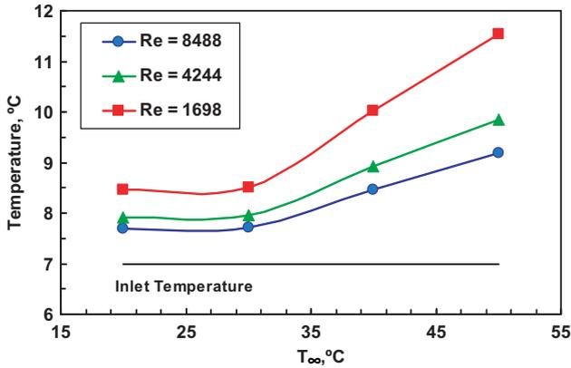
Fig. 9. Variation of the outlet temperature with the far-away temperature.
