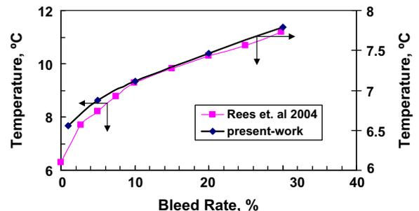
Fig. 14. The effect of bleed rate on the water outlet temperature for the present work and [10].
