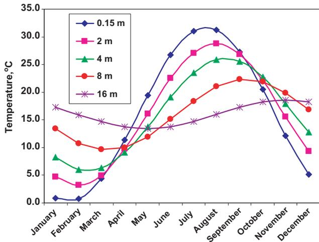
Fig. 3. The temperature distribution of the underground soil around the year for Queen Alia International Airport, Amman, Jordan.
