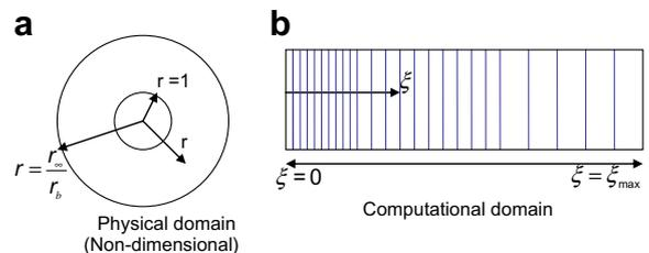
Fig. 5. Physical and transformed computational domain.
