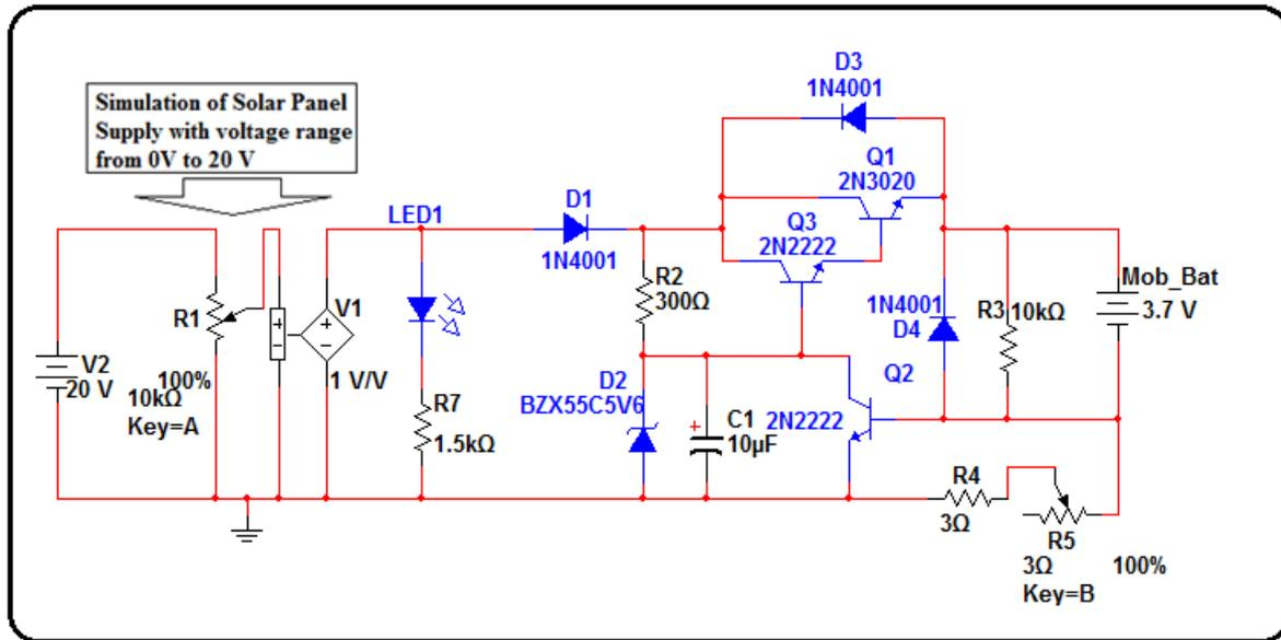
Fig. 1: The proposed electronic circuit of portable solar charger
