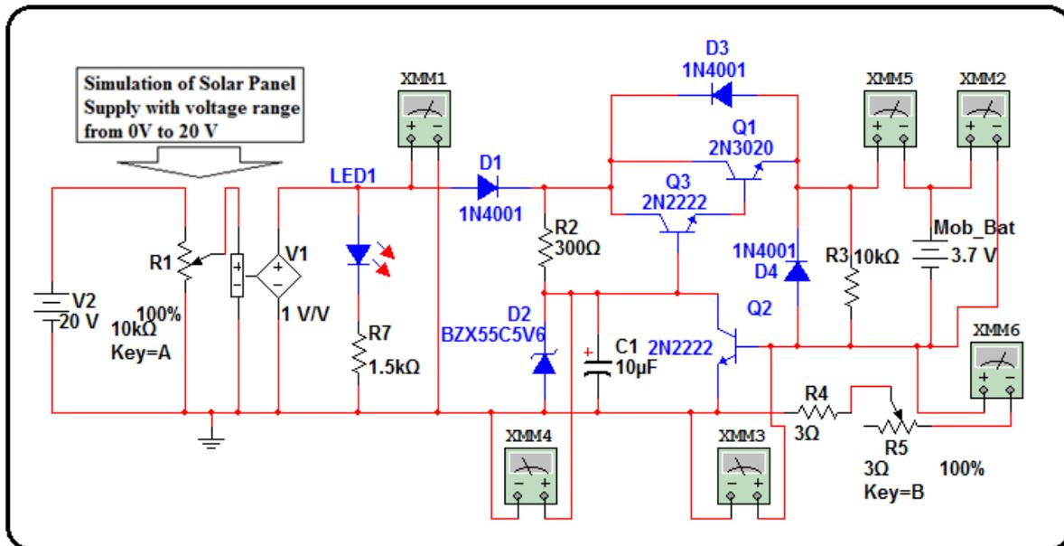
Fig. 2. The circuit of portable solar charger with voltage and current measurement probes
