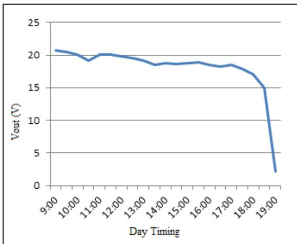
**Fig. 5: Open Circuit Output Voltages Day Timing of the Solar Panel Module / JBS-5W-12V**
