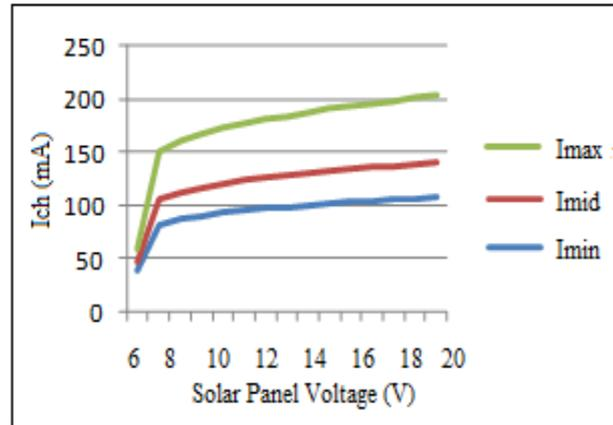
**Fig.3.: Charging Currents (mA) of mobile battery for different values of solar panel voltages.**
