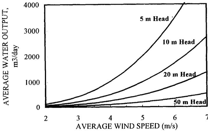
Fig. 4 Water output at different wind speeds and variable heights.
