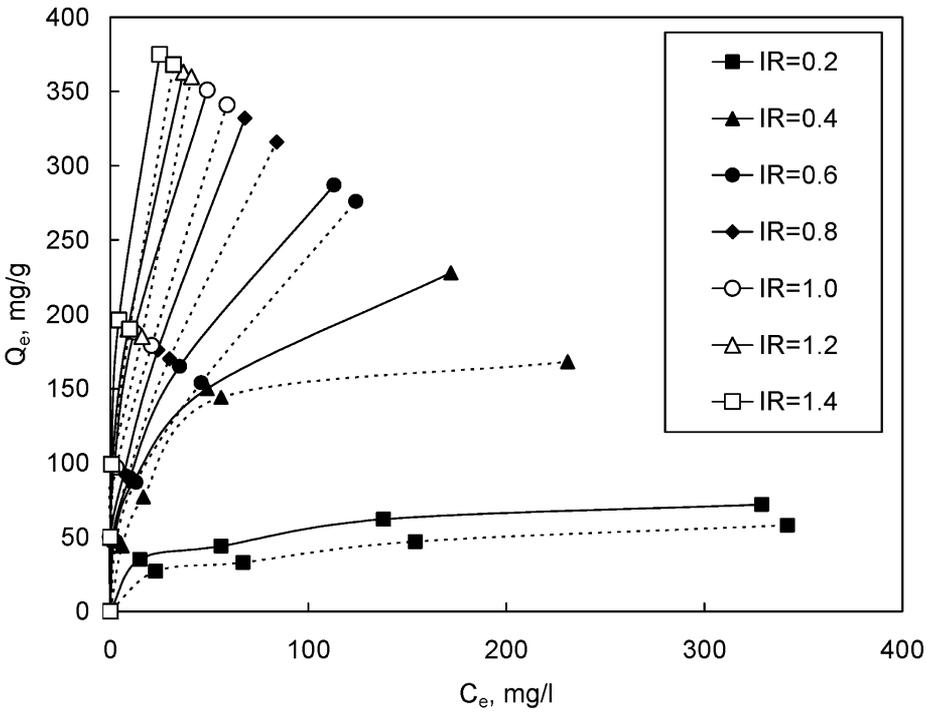
Figure 5. Effect of impregnation ratio on adsorptive capacity of methylene blue dye on activated product.
