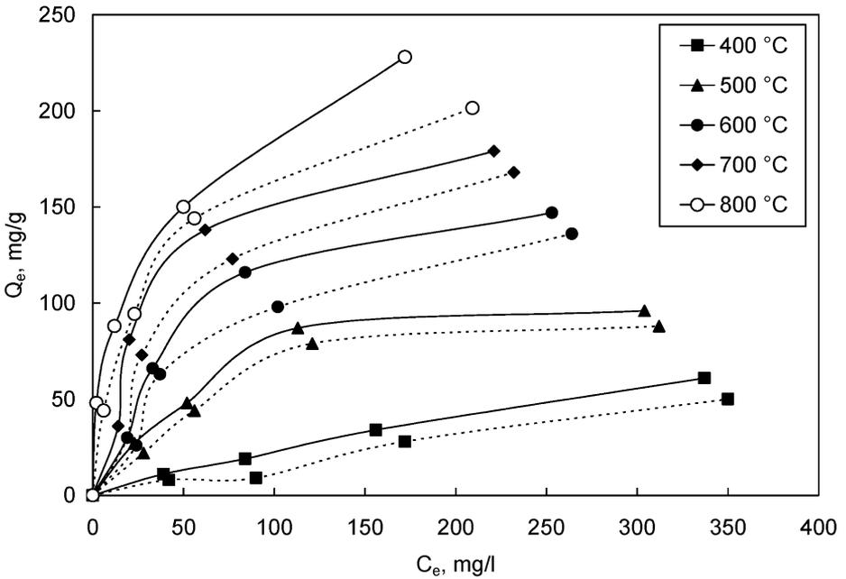
**Figure 4.** Effect of activation temperature on adsorptive capacity of methylene blue dye on activated product.
