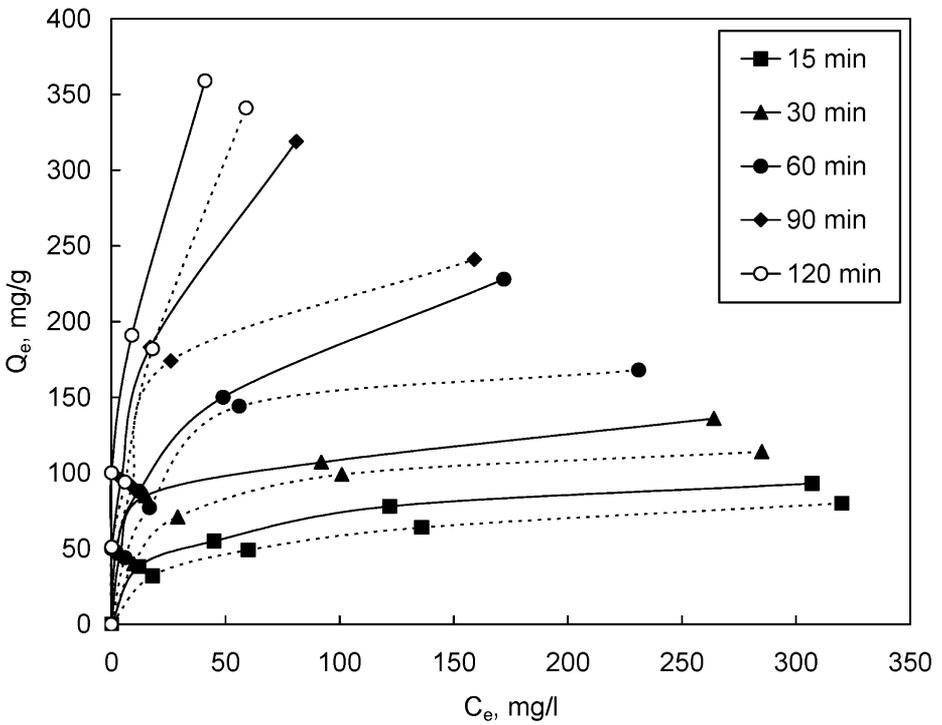
**Figure 2.** Effect of activation time on adsorptive capacity of methylene blue dye on activated product.
