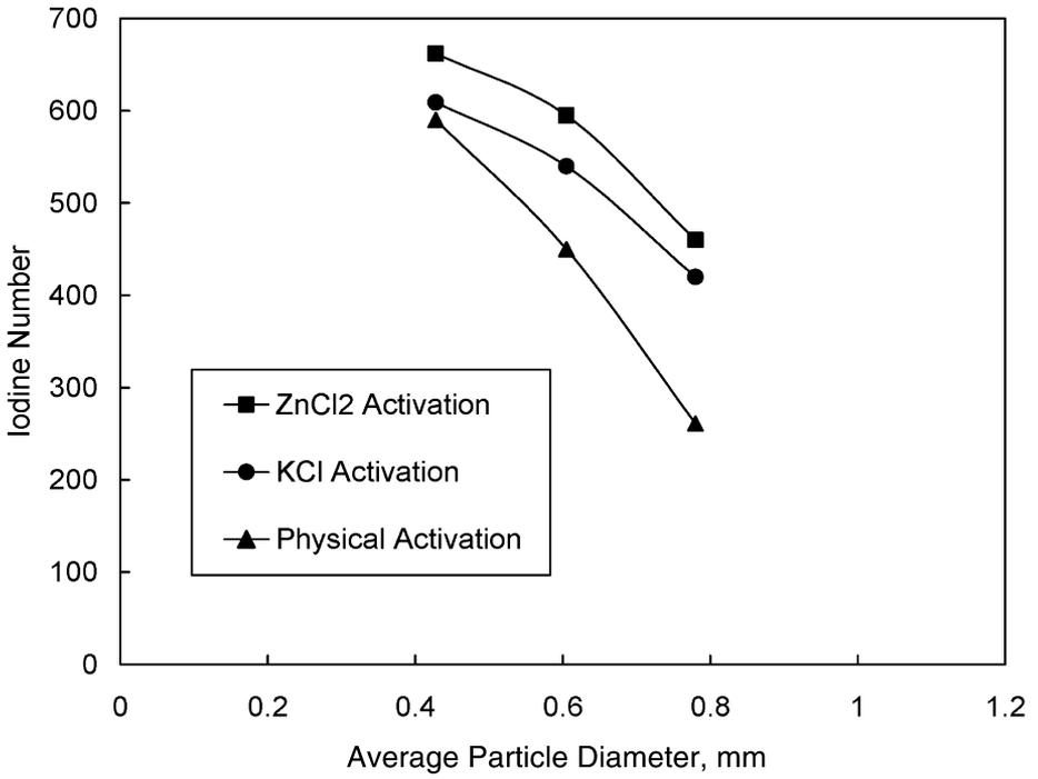
Figure 7. Effect of particle size on iodine number.
