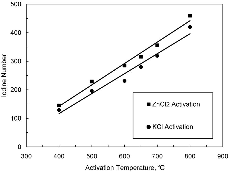
Figure 8. Effect of activation temperature on iodine number.
