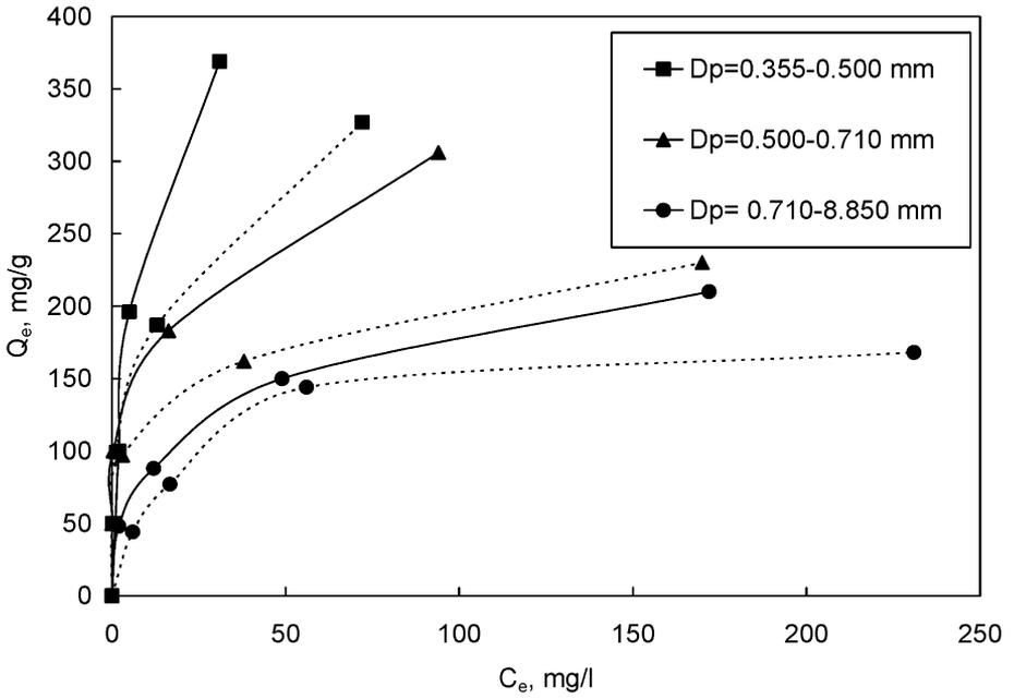
**Figure 3.** Effect of particle size on adsorptive capacity of methylene blue dye on activated product.
