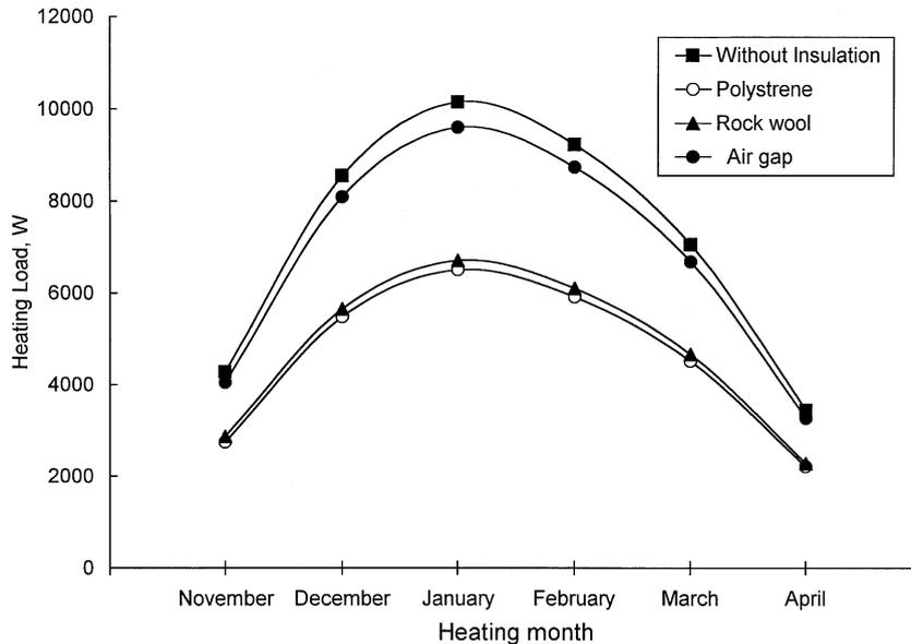
Fig. 9. Heating loads when wall insulation is used for the different materials.
