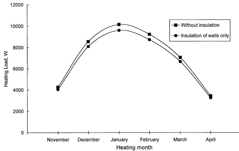
Fig. 8. Heating loads using air gap.
