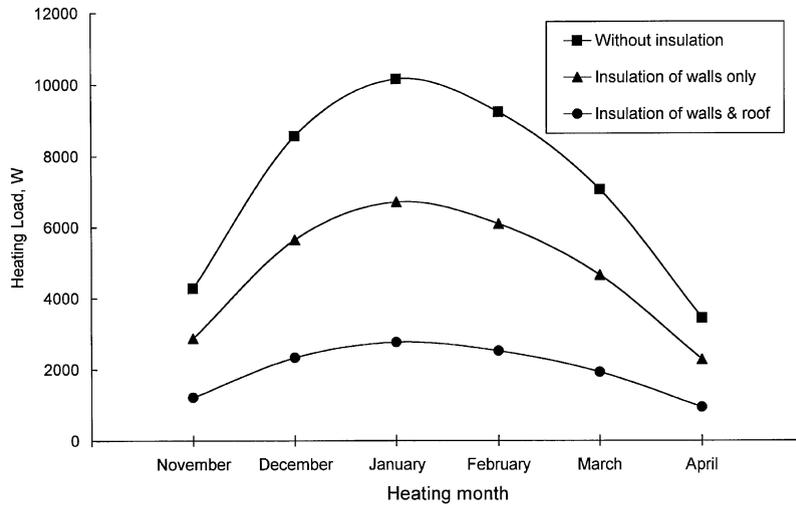
Fig. 7. Heating loads using rock wool.
