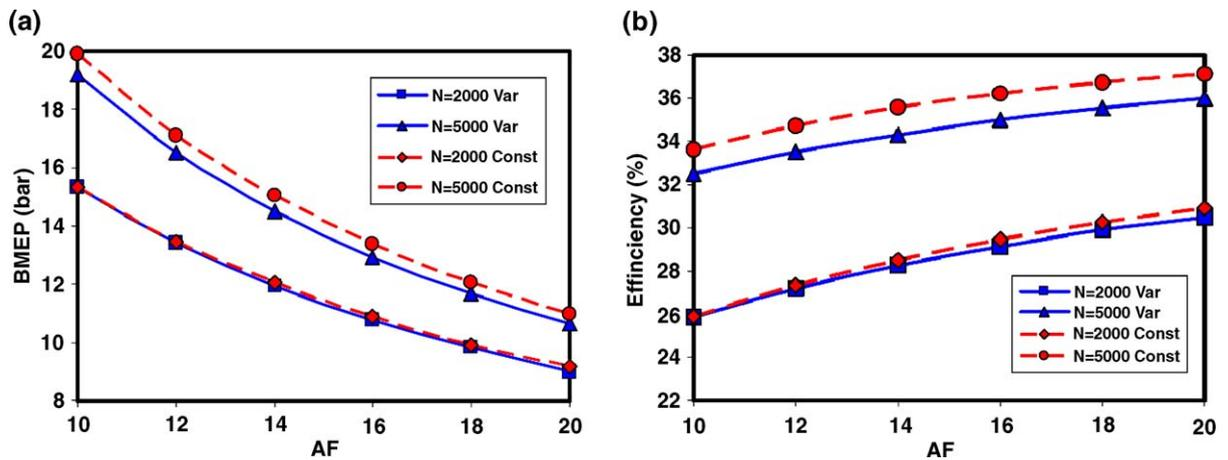
Fig. 6. (a) Brake mean effective pressure versus air–fuel ratio at different engine speeds using constant and variable specific heat models. (b) Efficiency versus air–fuel ratio at different engine speeds using constant and variable specific heat models.
