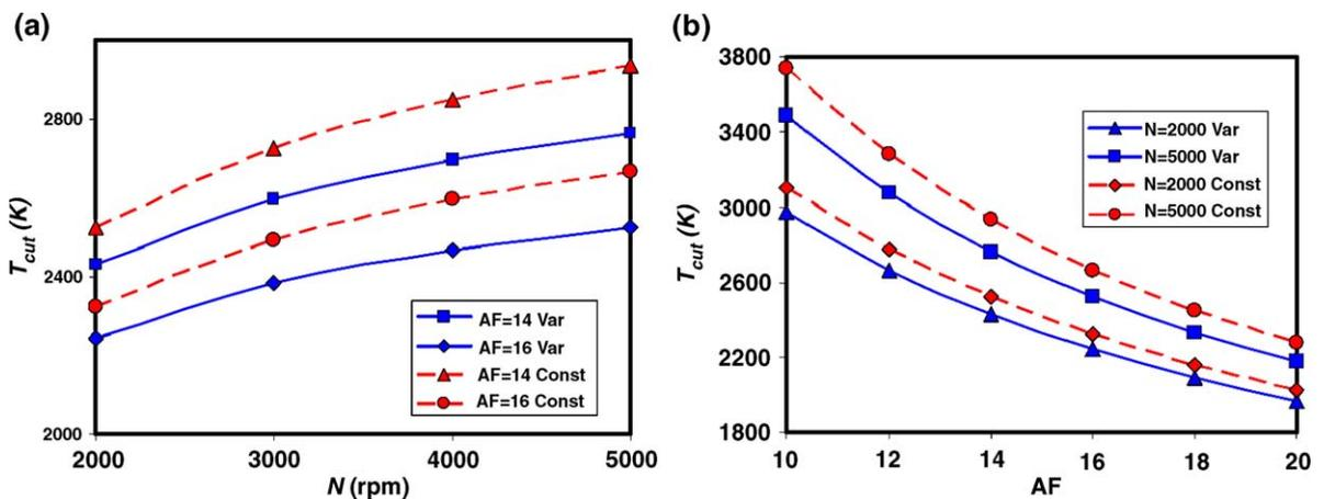
Fig. 5. (a) Maximum gas temperature versus engine speed at different air–fuel ratios using constant and variable specific heat models. (b) Maximum gas temperature versus air–fuel ratio at different engine speeds using constant and variable specific heat models.
