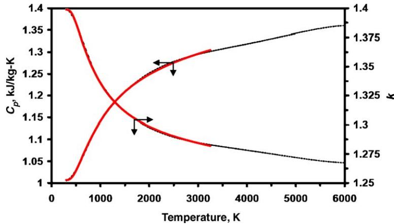
Fig. 1.  $C_p$  and  $k$  versus temperature for air (dotted lines representing Eqs. (1a) and (1b); solid lines representing Eq. (2)).
