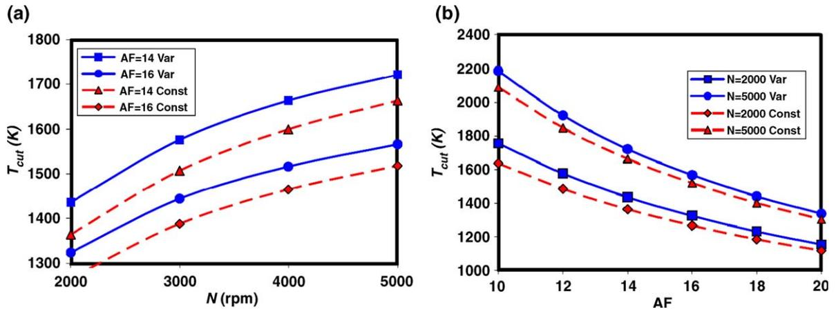
Fig. 4. (a) Outlet gas temperature versus engine speed at different air–fuel ratios using constant and variable specific heat models. (b) Outlet gas temperature versus air–fuel ratio at different engine speeds using constant and variable specific heat models.
