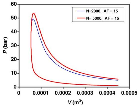
Fig. 2. Variation of cylinder pressure versus volume for SI engine using constant-specific heats running at 2000 rpm and 5000 rpm at air–fuel ratio of 15.
