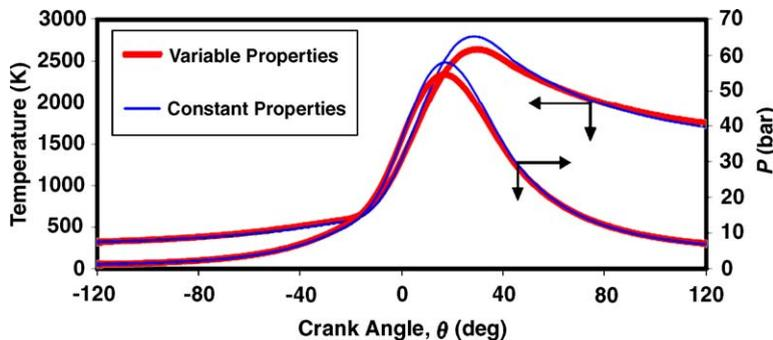
Fig. 3. Variation of gas temperature and cylinder pressure versus crank for SI engine using variable and constant-specific heats running at 5000 rpm and air–fuel ratio of 15.
