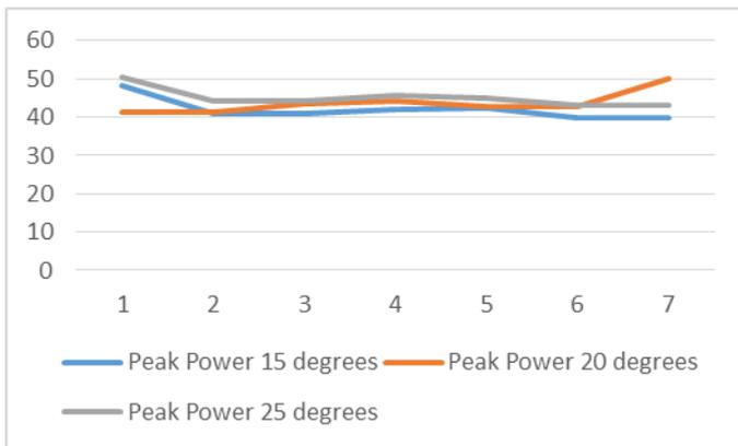
Figure 4. Peak power (Watt) with time (day index) for the three PV panels.
