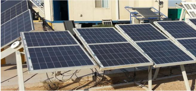
Figure 1. Experimental PV panels with different tilt angles.
