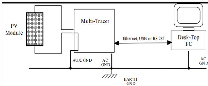
Figure 2. Connection of the multi-tracer.
