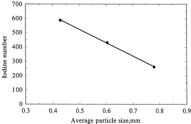
Fig. 11. Effect of particle size on iodine number for activation at  $800^\circ\text{C}$  and 60 min.
