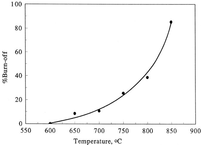
Fig. 3. Effect of activation temperature on percent burn-off for particle size 710–850  $\mu\text{m}$  and activation time 60 min.
