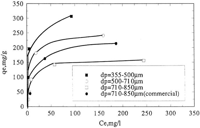
Fig. 10. Effect of particle size on adsorptive capacity at  $T_a = 800^\circ\text{C}$  and  $t_a = 60$  min.
