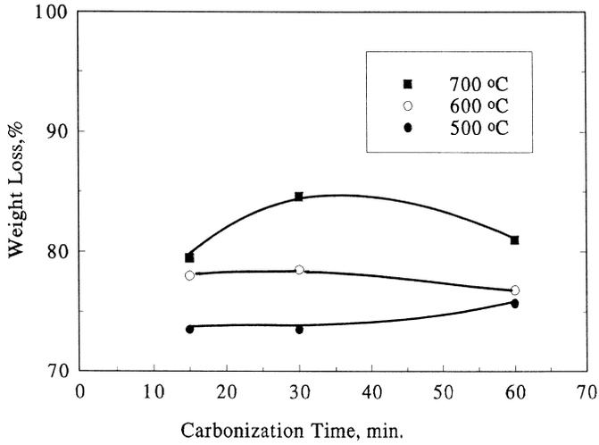
Fig. 2. Effect of carbonization temperature and time on weight loss for particle size 710–850  $\mu\text{m}$ .
