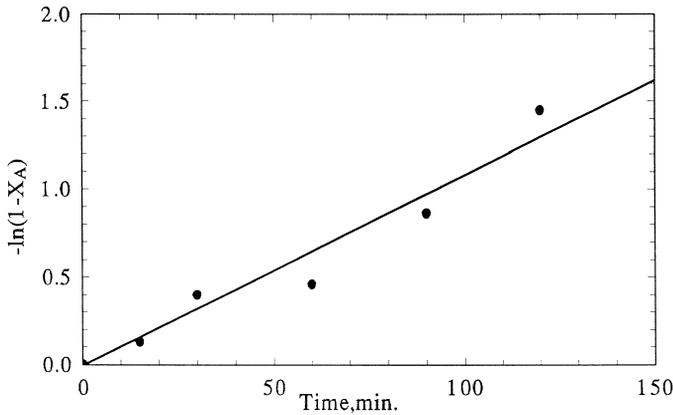
Fig. 12. Plot of  $-\ln(1 - X_A)$  vs. time for activation of olive-seed residue of  $d_p = 710\text{--}850 \mu\text{m}$  at  $800^\circ\text{C}$ .
