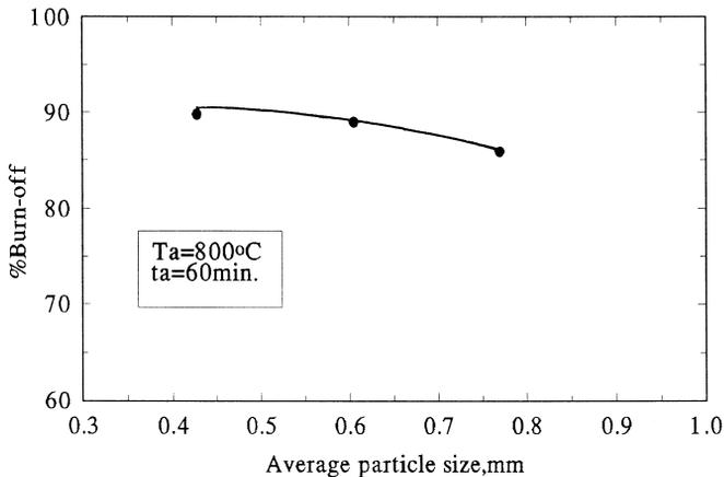
Fig. 9. Effect of particle size on percent burn-off for activation stage.
