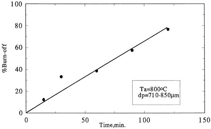
Fig. 6. Effect of activation time on percent burn-off of char.
