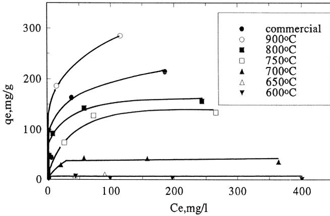
Fig. 4. Effect of activation temperature on adsorption capacity.
