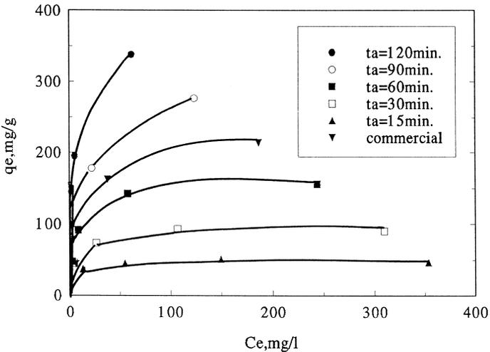
Fig. 7. Effect of activation time on adsorptive capacity for  $d_p = 710-850 \mu\text{m}$  and temperature 800°C.
