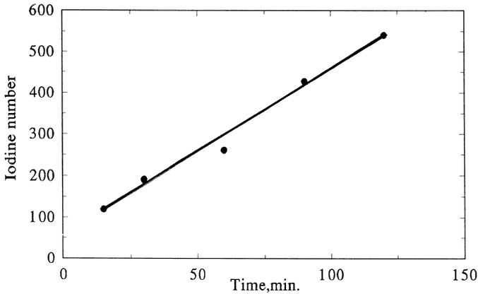
Fig. 8. Effect of activation time on iodine number for  $d_p = 710\text{--}850\ \mu\text{m}$  and temperature  $800^\circ\text{C}$ .
