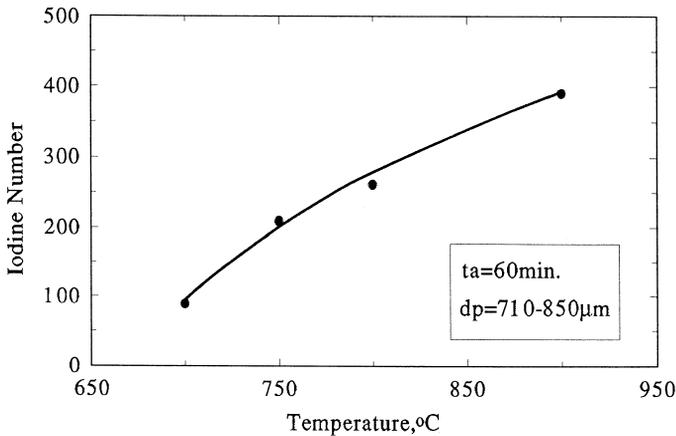
Fig. 5. Effect of activation temperature on iodine number.
