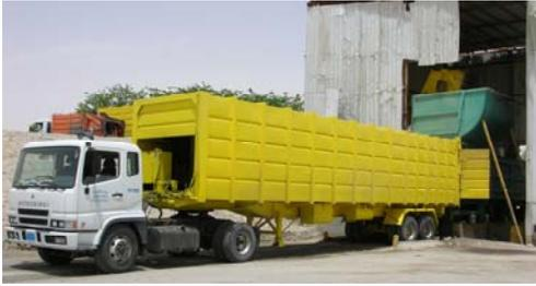
Fig. 6. A main hall truck (75 m<sup>3</sup> capacity)
