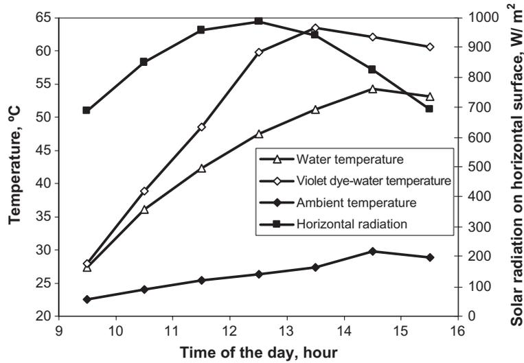
Fig. 5. Comparison of basin temperature for water–dye and water systems.
