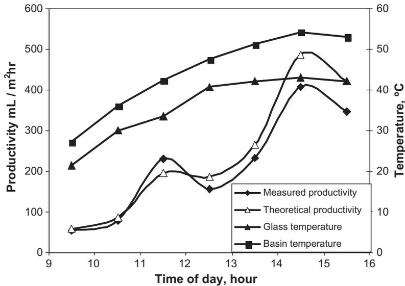
Fig. 4. Comparison of the theoretical and measured hourly productivities of the still.
