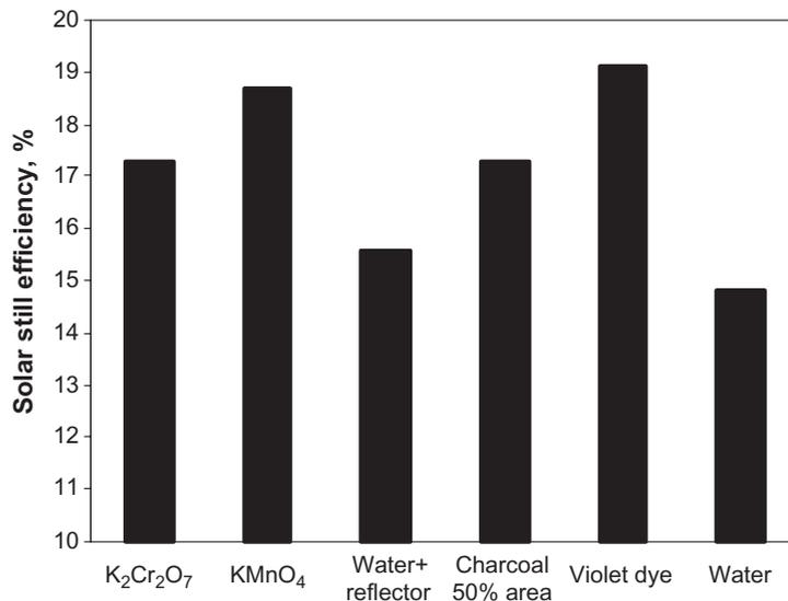
Fig. 2. Comparison of solar still daily efficiency using different absorbing materials.
