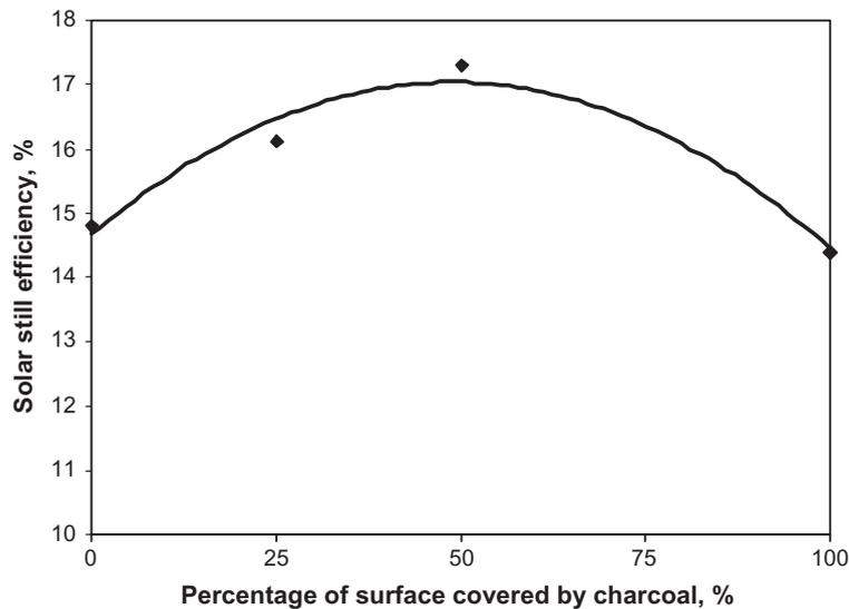
Fig. 6. Effect of proportion of the covered surface area by charcoal on efficiency of the still.
