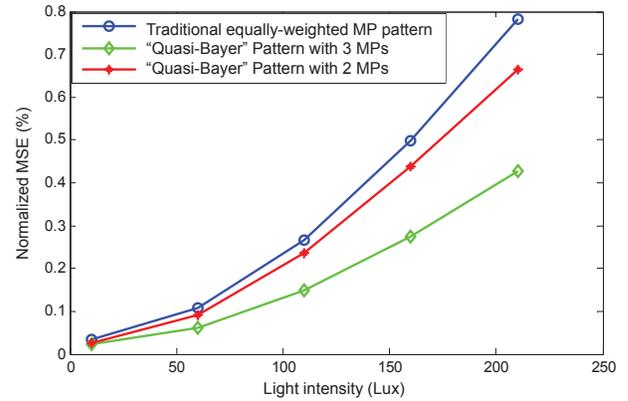
Fig. 6. The normalized MSE for different MP patterns.
