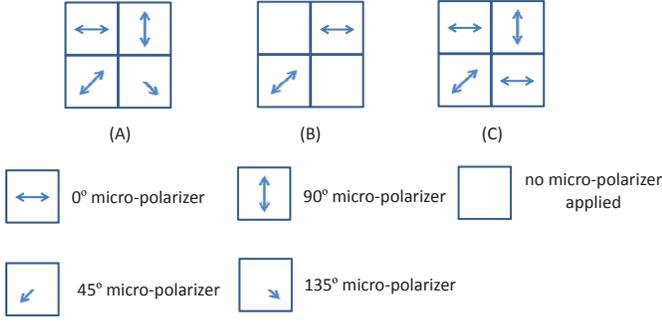
Fig. 1. Different MP patterns: (A) traditional equally-weighted MP pattern with four different micro-polarizers; (B) “Quasi-Bayer” patterns with two micro-polarizers; (C) “Quasi-Bayer” patterns with three micro-polarizers.
