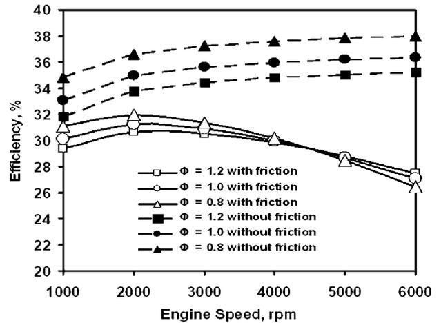
7 Efficiency versus equivalence ratio at different engine speeds using friction and no-friction models
