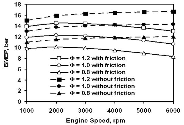
5 Brake mean effective pressure versus engine speed at various equivalence ratios using friction and no-friction models
