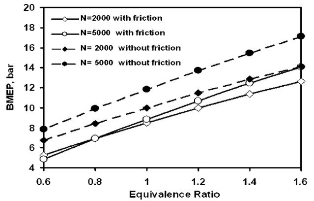
6 Brake mean effective pressure versus equivalence ratio at low and high speeds using friction and no-friction models
