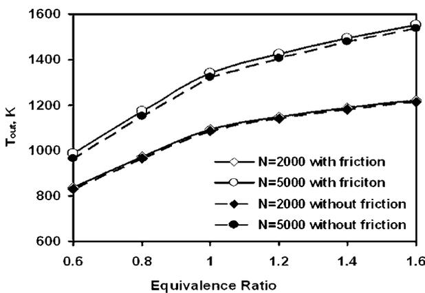
4 Outlet gas temperature versus equivalence ratio at low and high speeds using friction and no-friction models
