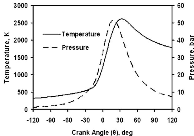
**2 Variation of gas temperature and cylinder pressure versus crank angle for SI engine using friction and no-friction models running at 3000 rev min<sup>-1</sup> and  $\Phi = 1$**
