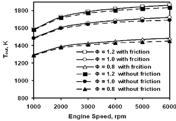
3 Outlet gas temperature versus engine speed at various equivalence ratios using friction and no-friction models
