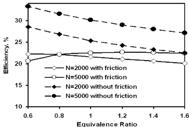
8 Efficiency versus equivalence ratio at low and high speeds using friction and no-friction models
