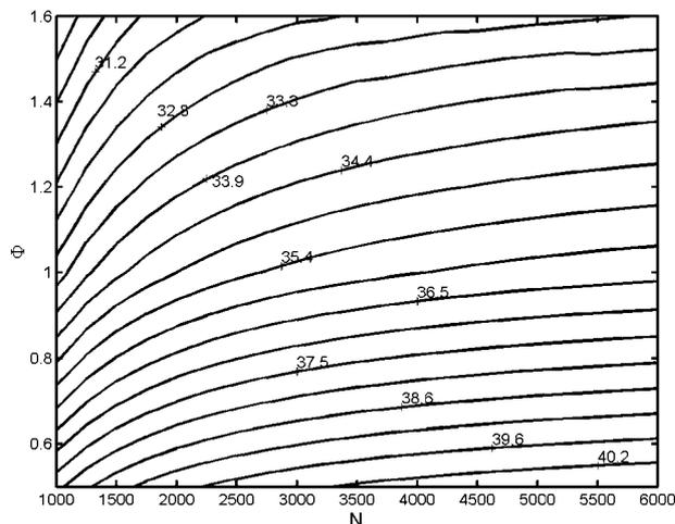
10 Contour plots for efficiency with no friction
