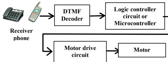
Fig. 1. System Block Diagram of DTMF Based Motor Pump Controller.
