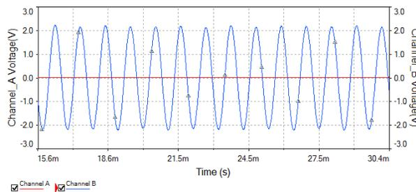
**Fig. 7. Output of Active Bandpass Filter for Frequency  $f_m = 941$  Hz.**
