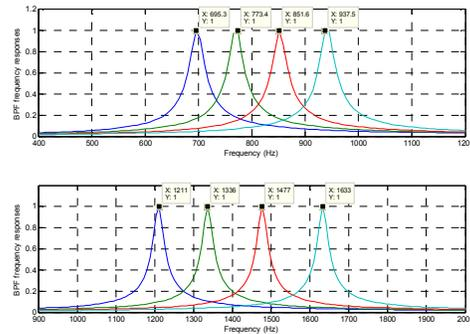
**Fig. 3: Magnitude Frequency Response of the Eight Digital Filters for Decoding DTMF Tones.**
