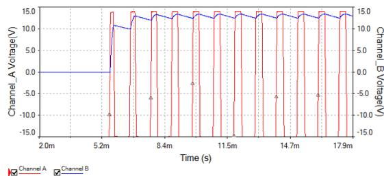
Fig. 9. A Comparator Output (Channel A) Integrator Output (Channel B).
