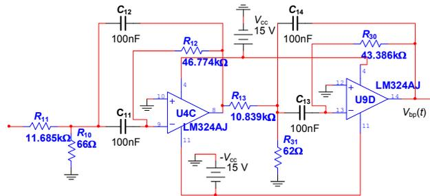
**Fig. 6. Fourth Order Multiple Feedback Topology Active Bandpass Filter (Component Values are for  $f_m = 941$  Hz).**
