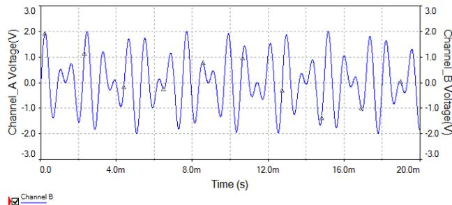
**Fig. 5. The DTMF Tone Corresponding to the Digit “0” at the Output of the Non-inverting Summer Shown in Fig. 4.**
