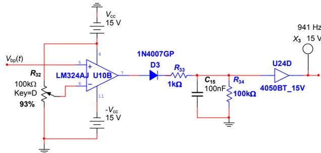
Fig. 8. A Comparator, Integrator and Buffer Circuit.
