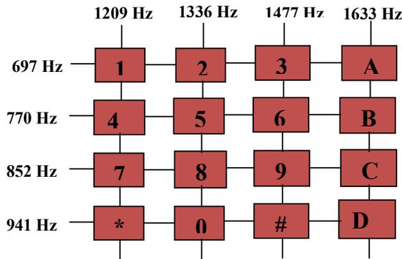
Fig. 2. The DTMF Tones Generated from a Phone Keypad.
