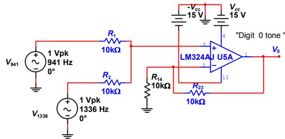
**Fig. 4. DTMF Tone Generating Circuit.**
