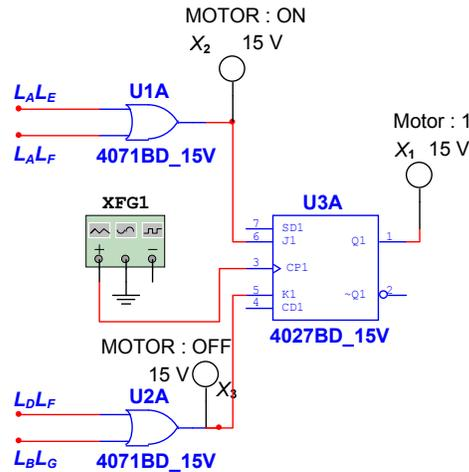
**Fig. 11. Controller Circuit for Motor 1.**
