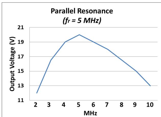
Figure 5: Behaviour of the parallel resonance LC Circuit
