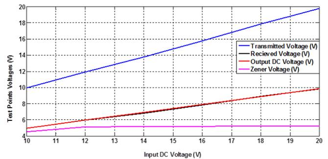
Figure 7: Stable Zener voltage during changing transmitted voltage value.
