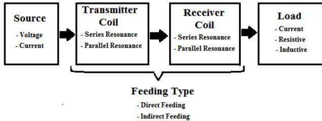
Figure 1: Overall block diagram
