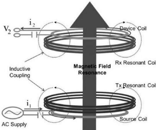
Figure 2: Indirect-fed wireless power transfer scheme [12].
