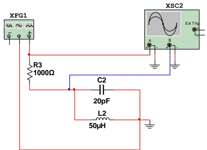
**Figure 3:** Designed LC circuit with resonance frequency 5 MHz
